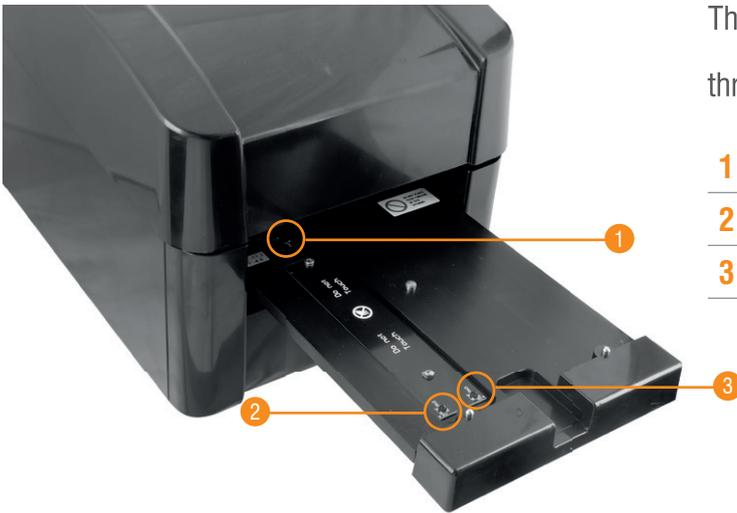
The trayflex contains PCB card on it which there are placed three sensors:
